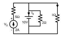
Q.50 The current in the  $1\Omega$  resistor in Amps is
